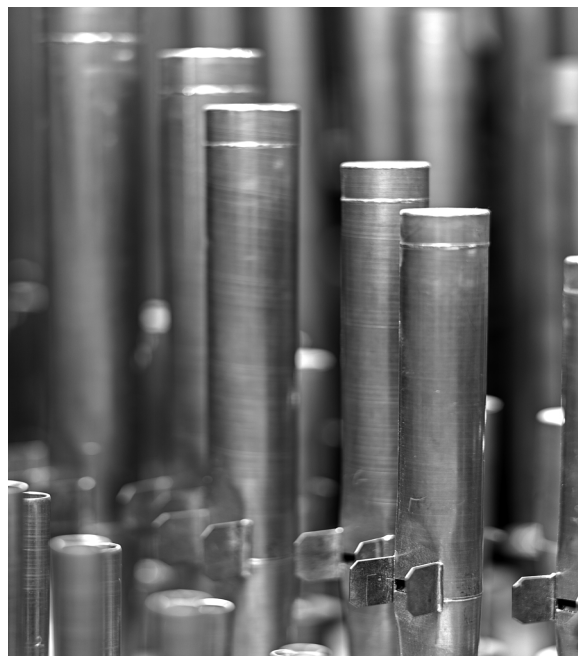
The Quintadena pipes with soldered tops and tuning ears
