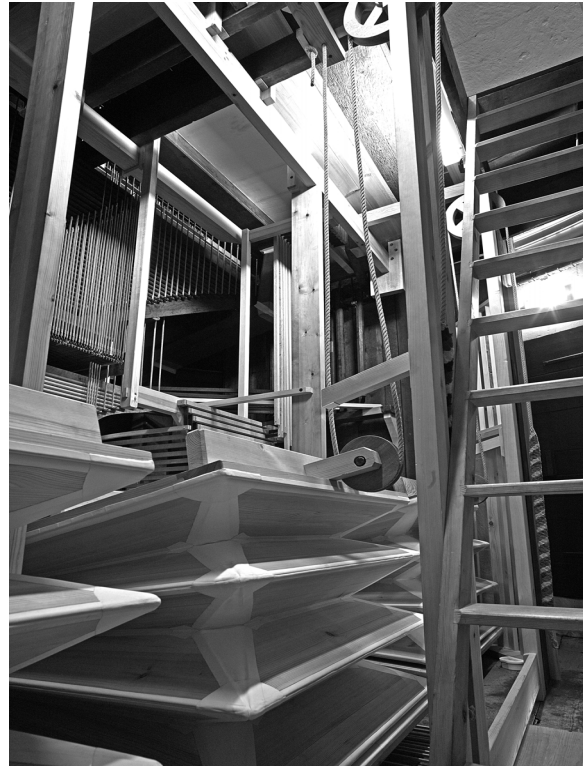
The organ: bellows with motor switched on
