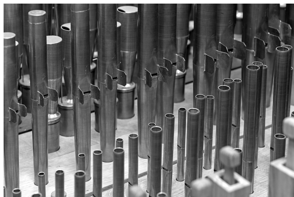
The characteristically low cut-ups from which the Quintadena pipes get their unusual sound.
