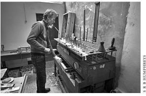
Above: Joost de Boer regulating some of the original flue pipes on the voicing machine
