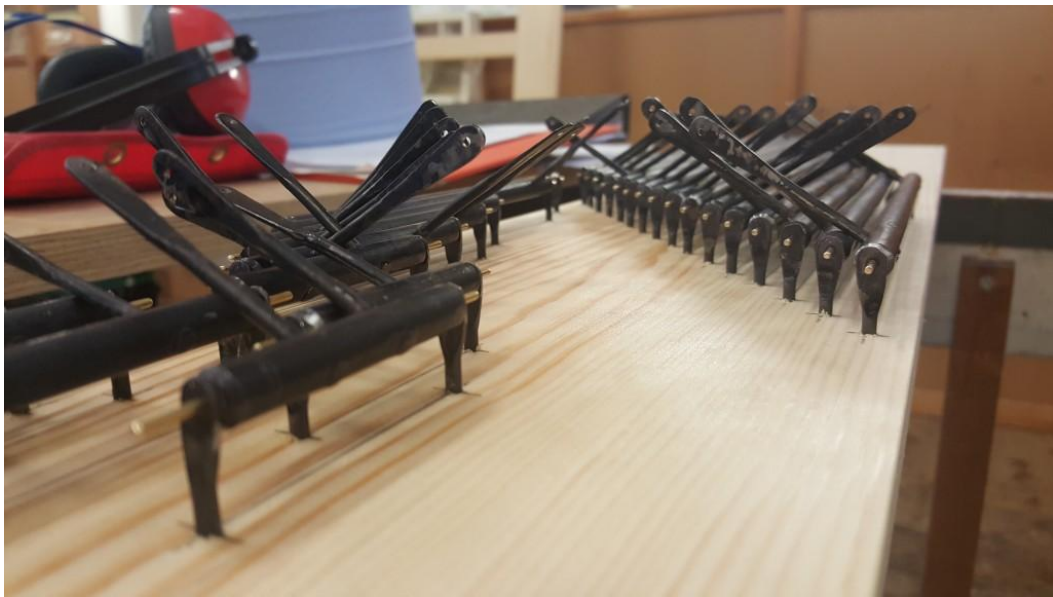
New metal-roller, which made in William Drake's Ltd workshop.
