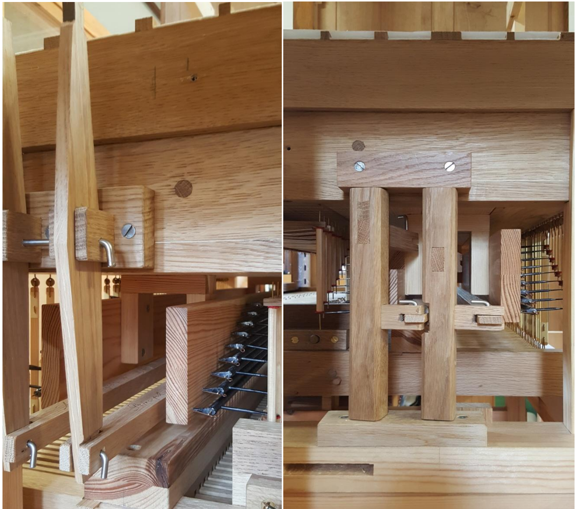
Stop Action in organ of Westminster Abbey Song School. (L) Rocking Lever, (P) Trundles. As we can see, all the parts of the stop action are made by the hardwood-oak, and connected by means of the iron rods.
