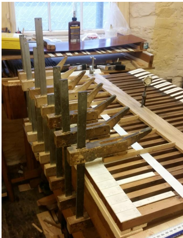
Gluing and carefully clamping the bone cover using the hot glue
