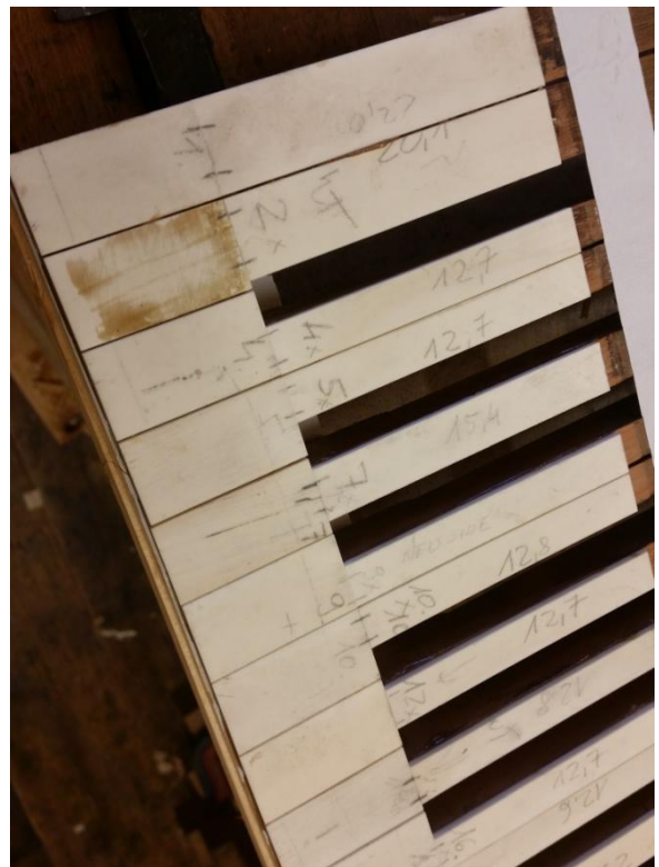
Gluing and carefully clamping the bone cover using the hot glue
