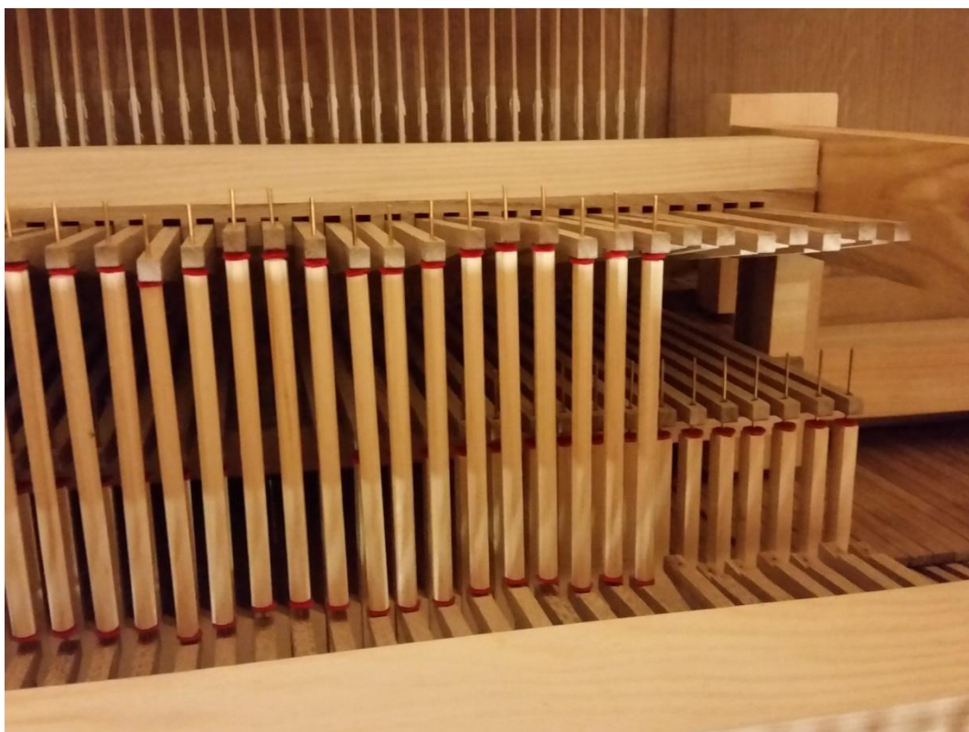
Two new backfalls are connected by the square stickers, while the keyboard tails are connected by rounder stickers with third backfall.
