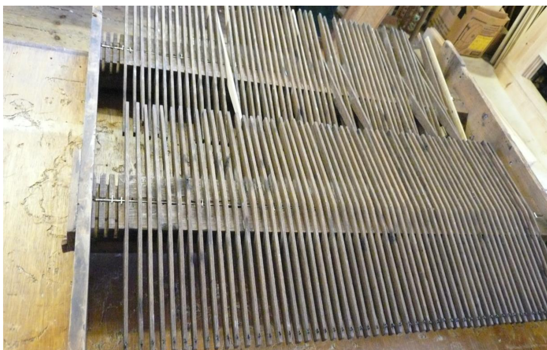
Original double backfall by Richard Bridge organ from 1735. The Christ Church Spitalfields, London.
