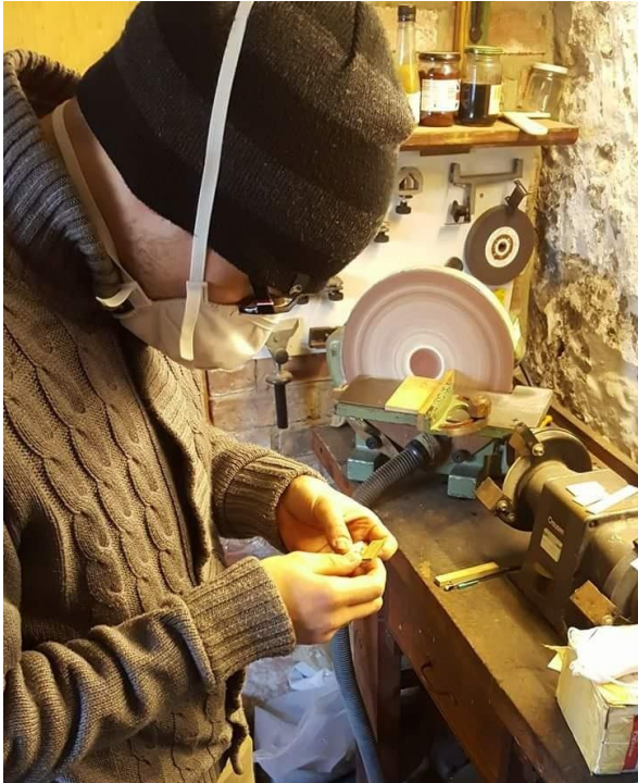
Grinding bone key covers to size:
